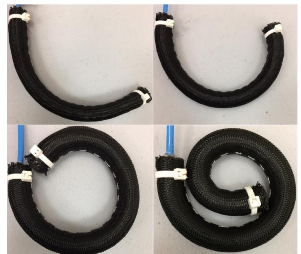
Fig.10. Various pressure levels pressurize BEPAM [29].
