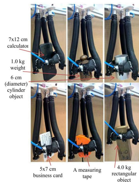
Fig.27. The circular gripper with extension may hold many objects [40].
